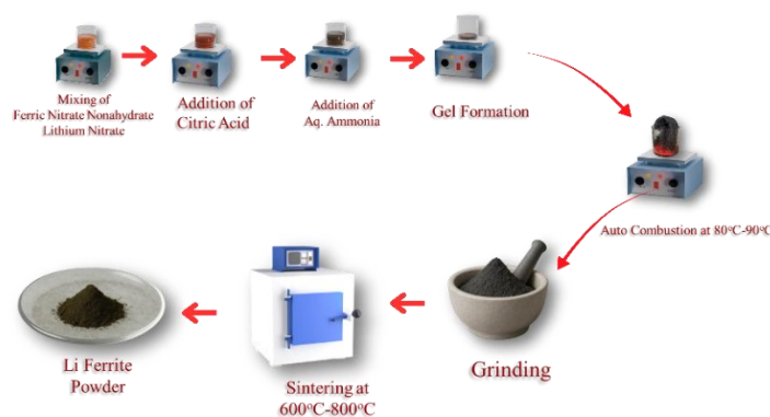
Fig 2: Synthesis of Lithium Ferrite By sol-gel route
